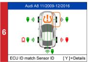
Green signal and OBD icons: the ECU ID matches Sensor ID. Red signal and OBD icons: the ECU ID does not match
