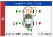
Read sensor ID from ECU, check sensor ID matching condition, read DTCs from TPMS ECU and clear DTCs
