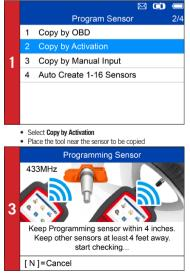
· Place a new MX-Sensor near the top of the device to program
