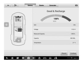
Figure 17-6 Sample Battery Test Results Screen
