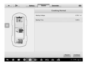
Figure 17-7 Sample Starter Test Result Screen
